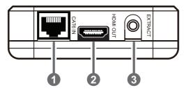
**CAT6 IN Port:** Connect to a compatible Cat.6 transmitter with a single Cat.6, or better, cable for reception of all data signals. Power via PoC is also supplied to this unit by the connected compatible PSE transmitter.
