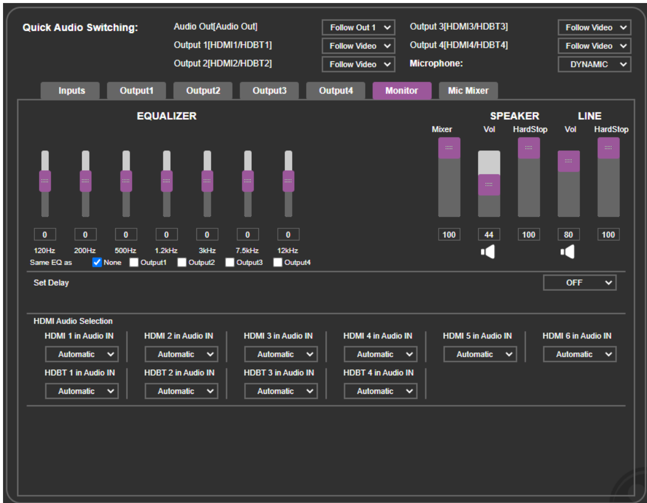
Figure 30: Audio Settings Page – Setting the Monitor and Speaker Outputs
