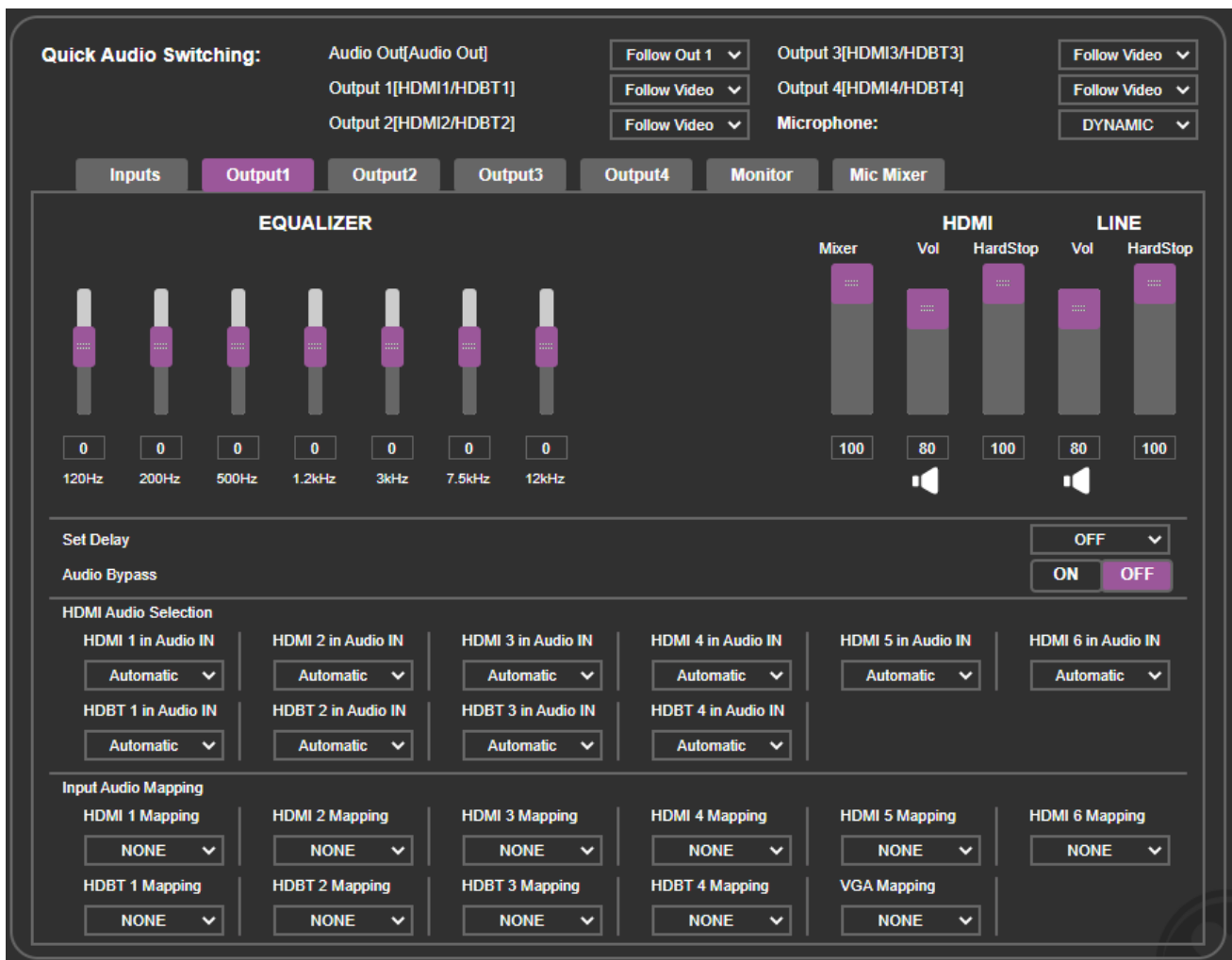
Figure 29: Audio Settings Page – Setting the Audio Outputs
